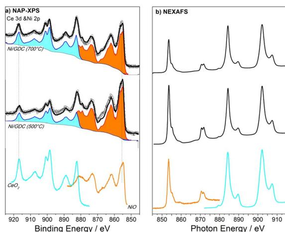
**Figure 1.** a) Ce 3d/Ni 2p ( $h\nu = 1065$  eV) NAP-XPS spectra. b) Ni  $L_{3,2}$ - and Ce  $M_{5,4}$ -edge NEXAFS spectra. The measurement conditions were 0.2 mbar  $O_2$  at 700 (top) and 500 °C (middle). The measured Ce 3d/Ni 2p spectrum ( $\circ$ ) is well fitted ( $—$ ) by a linear combination of the reference  $CeO_2$  and NiO spectra (bottom) measured from standard powder samples under similar acquisition conditions.
