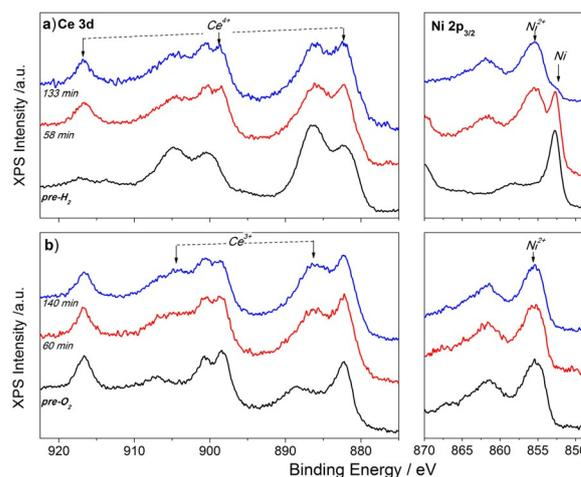
**Figure 3.** a) Ce 3d and Ni 2p $_{3/2}$  ( $h\nu = 1065$  eV) NAP-XPS spectra for the NiGDC electrode recorded at 700 °C after various H $_2$ O exposure periods; a) electrode pretreated in H $_2$ , b) electrode pretreated in O $_2$ .
