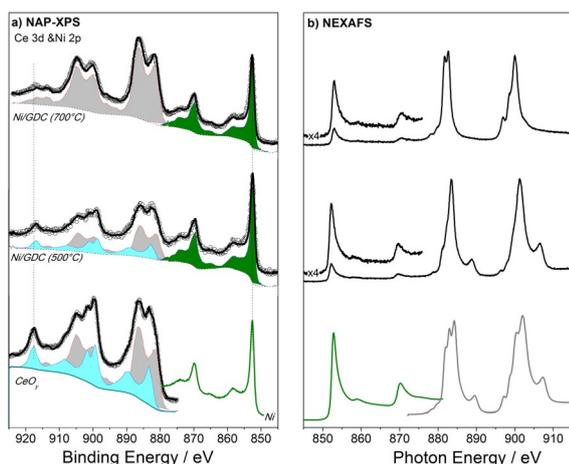
**Figure 2.** a) Ce 3d/Ni 2p ( $h\nu = 1065$  eV) NAP-XPS spectra b) Ni $L_{3,2}$ - and Ce $M_{5,4}$ -edge NEXAFS spectra. The Ni $L_{3,2}$ -edge is magnified four times. The measurement conditions were 0.2 mbar H $_2$  at 700 (top) and 500 °C (middle). The measured Ce 3d/Ni 2p spectrum (○) is well fitted (—) by a linear combination of the reference CeO $_{1.5}$  and metallic Ni spectra (bottom) measured from standard powder samples under similar acquisition conditions.
