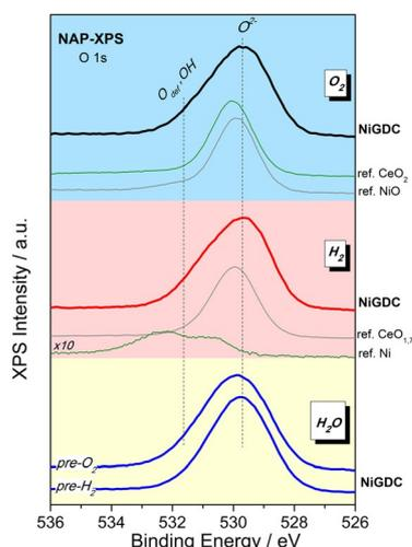
**Figure 5.** O 1s ( $h\nu = 710$  eV) NAP-XPS spectra recorded at 700 °C in O<sub>2</sub>, H<sub>2</sub>, and H<sub>2</sub>O atmospheres (from top to bottom) for NiGDC (—) and reference nickel and ceria powder samples (---).
